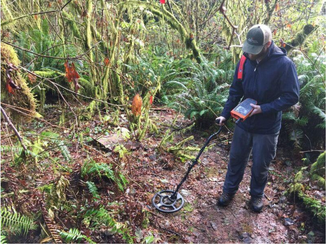
Figure 5. Scanning the plot established in the angiosperm understory of the Redwood Experimental Forest in Klamath, CA. Equipment featured include an HP Plus PIT tag reader connected to a BP Plus portable antenna; together they can be used to scan large areas for fossorial, PIT tagged animals.
