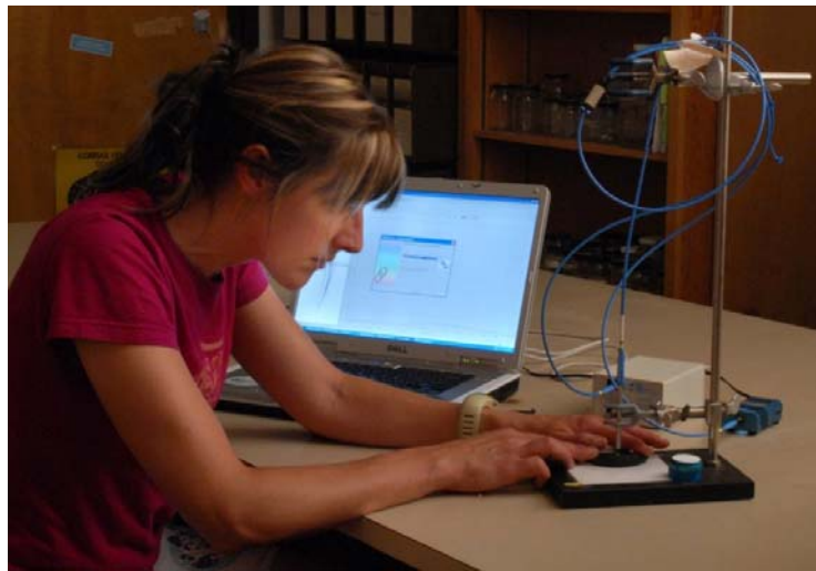
Figure 4. Photograph illustrating how spectral measurements were collected in the laboratory. Spectrophotometer and light source are shown in the background (far right) with the reflectance probe leading from those units to the sample (i.e. snake or habitat sample) situated on the platform. The position (angle and distance) of the reflectance probe was maintained constant by holding the probe in place with clamps on the stand. All data are collected using the SpectraSuite program (Ocean Optics) shown on the computer.
