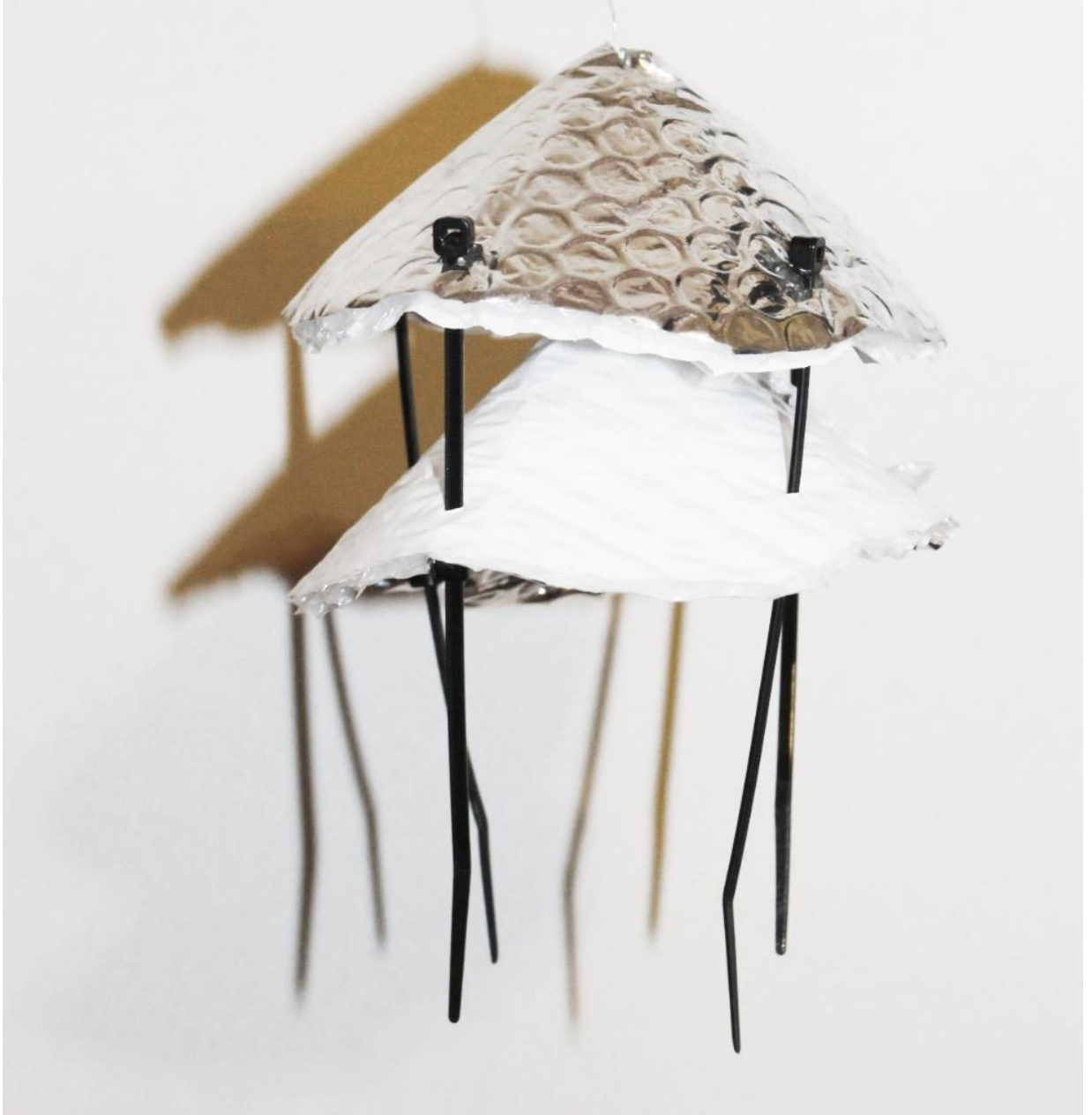
Figure A 1. A prototype of a double cone used for air temperature loggers. Distance between top and bottom cone edges is 3-5cm. An air logger was placed inside the top cone secured in a plastic Ziploc bag. Cone design was adopted from literature (Tarara and Hoheisel 2007).
